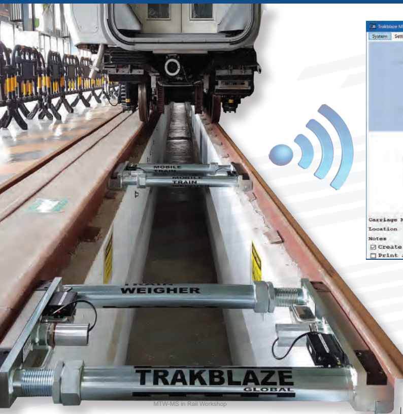
Standard PC software displays and records all the weighing results
