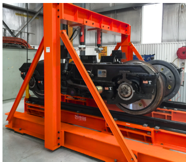
Bogie balancing press fitted with TRAKMATE loadcells
