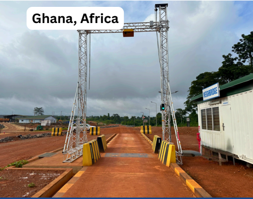
FORCE 1 with the traffic lights stop/go and our TVS truck volumetric scanner
