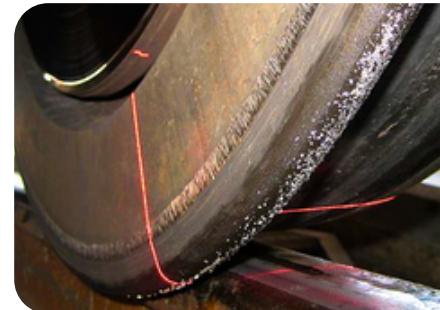
Apart from the typical wheel parameters, the following flange defects can be measured by the Wheel Pro, (limits to be specified by the customer):
