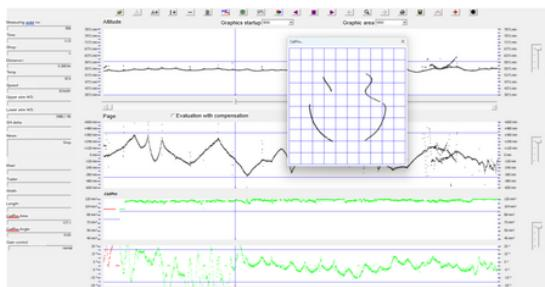
The CatPro Viewer software allows users to compare routes over time to forecast areas of wear. It also enables the export of measurement data in standardised formats for integration with route management systems.
