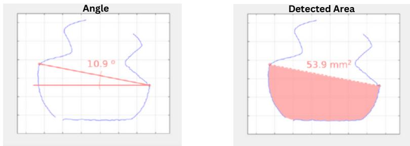
The system detects the relevant area of the contact wire.
