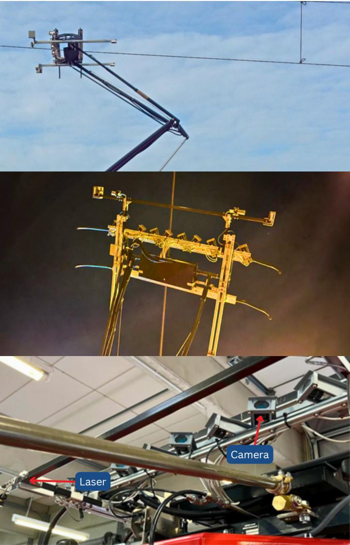
The **CatPro** optical contact wire wear measurement system continuously monitors wear on the contact wire during operation. Even while the contact voltage is active it provides crucial support for overhead line maintenance. Unlike traditional measurement methods, CatPro significantly reduces both the manual effort required and the distance between measurement points is greatly reduced offering a more efficient and streamlined process.
