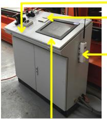
Touch screen PC controller displaying wheel loads & applied
