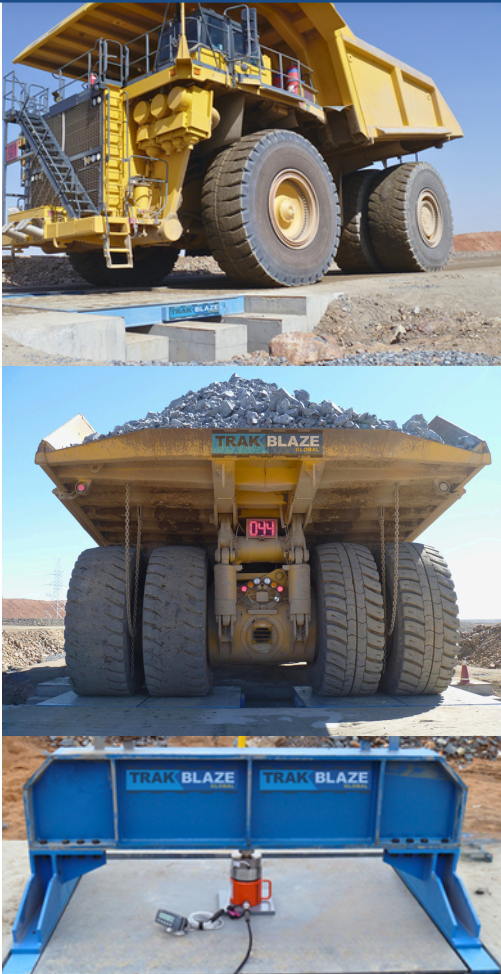
FORCE being tested and calibrated at site with a portable test press unit
