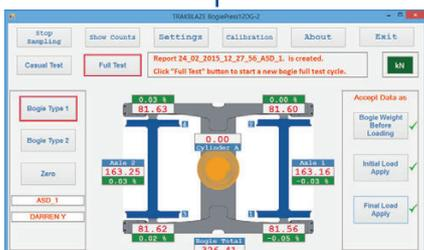
Touch screen PC controller displaying wheel loads & applied
