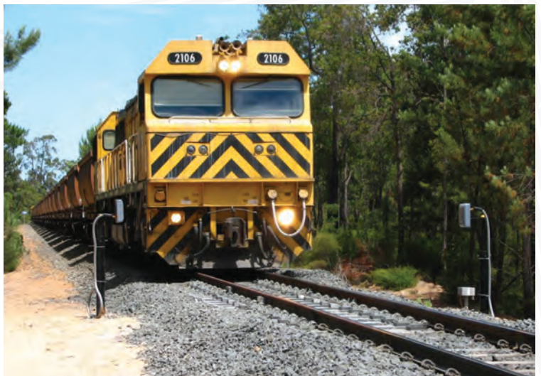
Installed INFINITY 'HS' weighing system with (optional) tag readers
