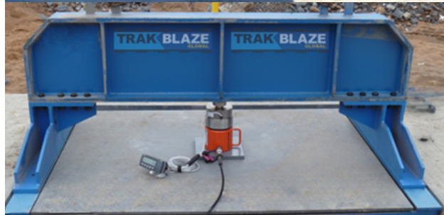
FORCE being tested and calibrated at site with a portable test press unit
