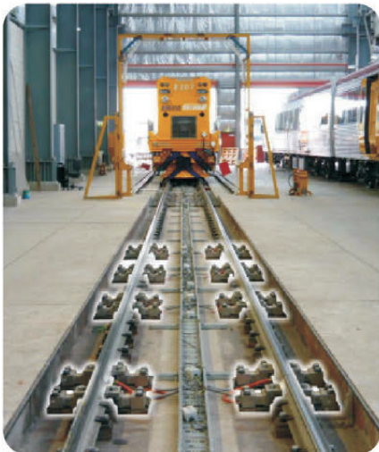
Trakmate 2 loadcells under rails
